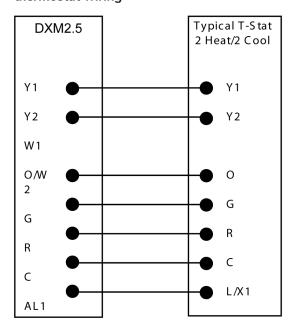
NOTE: For units with two (2) DXM2.5 boards all thermostat connections will be made to the "Master" DXM2.5 board. DO NOT connect thermostat wiring to the "Slave" DXM2.5 board.
