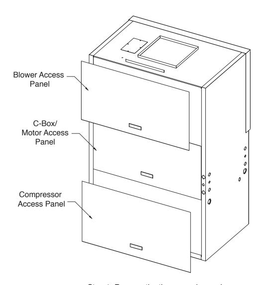
Step 1: Remove the three panels, as shown.
