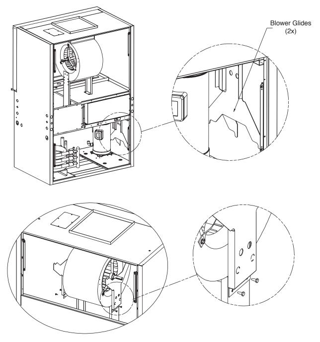
Step 5: Attach Blower Glides to Blower BTM Load Brackets as shown. Use bottom set of holes (.203 Dia.) on Blower BTM Load Brackets. Blower Shaft should be sitting right on top of the Blower Glides.
