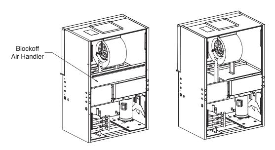
Step 3: Remove bolts (4x) off blower panel. Remove bolts (4x) (2x ea. side) from blower sides.
