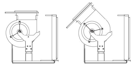
Step 8: When the Blower ASM is parallel to the floor, push the Blower ASM back so that the Blower Panel is flush with the unit.
