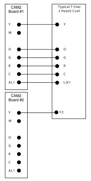
Figure 13b: Typical Manual Changeover 2 heat/ 2 cool thermostat wiring
