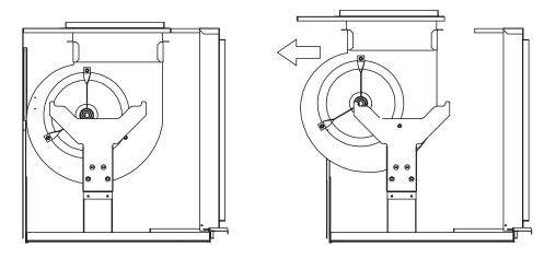
Step 7: Rotate Blower ASM using Blower Glides as a guiding track.
