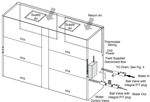
Figure 4: Typical Water Loop Application
