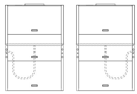
Installer will untie flex hose and make an internal trap on either the left side (shown above) or on the right side. Internally attach mounting plate with FPT fitting.
