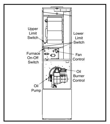
Figure 28. Furnace Controls - Oil Furnace
