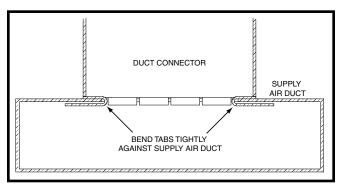
Figure 10. Duct Connector Tabs
