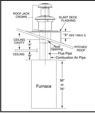
Figure 16. Ceiling Cavity Depth
