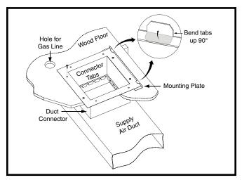
Figure 8. Standard Duct Connector Installed
