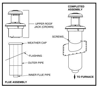
Figure 23. Roof Jack Crown
