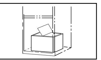
Figure 29. Coil Cavity Damper
