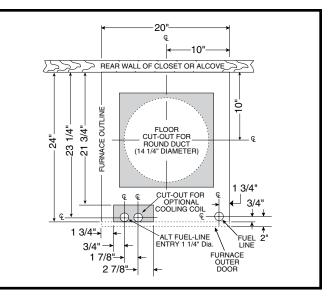
Figure 7. Cut-Out Dimensions for Round Duct Connectors
