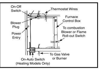
Figure 24. Control Panel (All Models)
