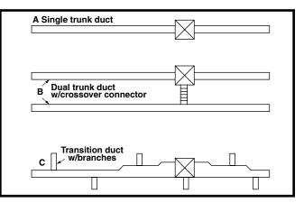
Figure 5. Typical Supply Duct System
