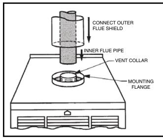
Figure 22. Combustion Air Pipe Connection
