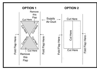
Figure 11. Narrow Air Duct Openings
