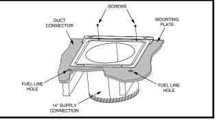
Figure 13. Round Duct Connector Installed
