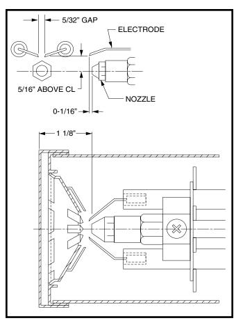
Figure 27. Oil Gun electrode Position
