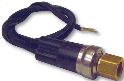
When the pressure in the system exceeds the high pressure switch setting, the switch will open circuit the compressor clutch and the compressor will stop circulating refrigerant. The high pressure setting of the switch must correspond to the type of refrigerant in the system. Different refrigerants require different settings.
